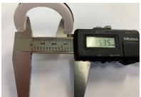
c. Measure Outside diameter of stationary over O ring or boot
