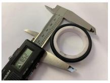
e. Measure Internal diameter of Rotary
