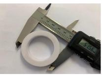
d. Measure height (width/ thickness)
