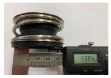
NOW measure compressed and uncompressed height of rotary on old seal
